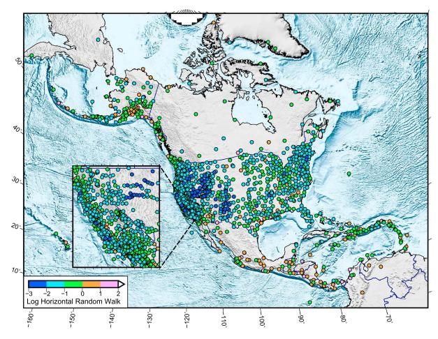
Figure 12. A measure of the temporal correlations in the time series based on the estimates of the process noise random walk variances for the site horizontal position residuals. Values are shown as log(mm<sup>2</sup>/yr).
