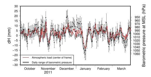
**Figure 19.** Example of height variations due to atmospheric pressure loading for site AB15. The observed GPS time series is shown by the black dots with one standard deviation error bars. The range of daily observed barometric pressure at a nearby meteorological station is shown in gray. The equivalent atmospheric load, calculated from the IERS geophysical fluids center and referenced to the center of figure frame [see *Blewitt*, 2003], is shown by the red line.
