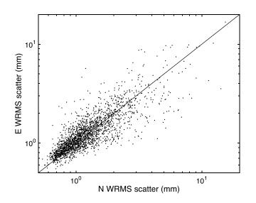
**Figure 10.** Log-log plot of the north and east WRMS scatter of the 2137 stations in the GAGE analysis of data collected between 1996 and the end of 2015. The solid line shows a one-to-one correlation.
